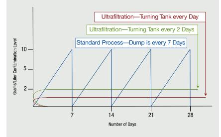
Figure 2: Comparison of contamination levels in a typical aqueous cleaning system and a cleaning system with UF.
